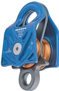
Dual Sheave, swing cheek pulley with a full strength central becket. Prusik minding design allows for progress capture. Now compatible with 13mm ropes.
